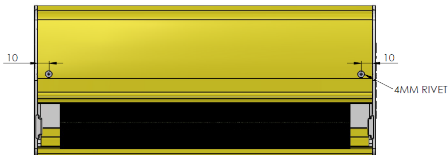
Bottom view of the 2-part pelmet with front fixing using rivets
