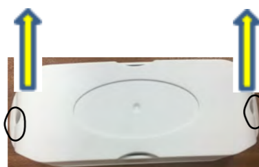
Remove two screws by screwdriver
